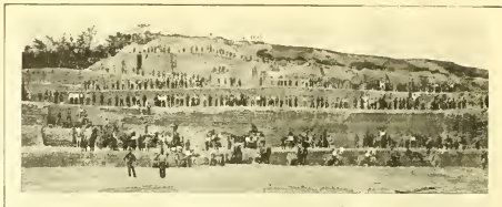
Clay beds at Roseton, New York. Notice the manner of quarrying the clay from successive terraces, thus accommodating a great many laborers at one time.
